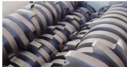
Figure 1.6 Rotary-Shear shredder used for RDB production
