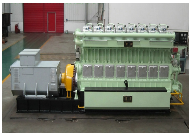
Figure 27: Medium-Speed IC Engine, designed for operation with Low-BTU fuel-gas
