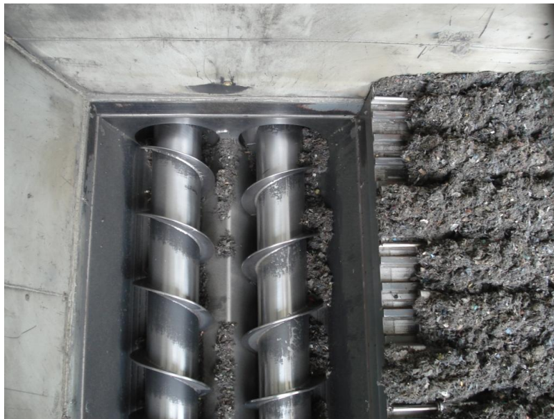
Figure 71: Walking Floor Storage Controls RDB Feed Rate to Gasifier
