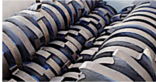
Figure 70: Rotary-Shear shredder used 2-stage Size-Reduction and for RDB production
