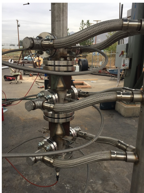
Figure 50: Pulse-Detonation Installed on the bottom of the JSB
