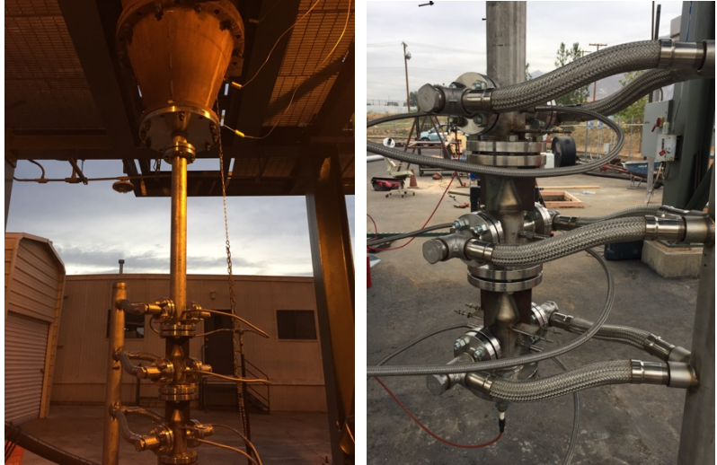
Figure 11: Detonation-Burner Firing into Jet Spouted Bed
