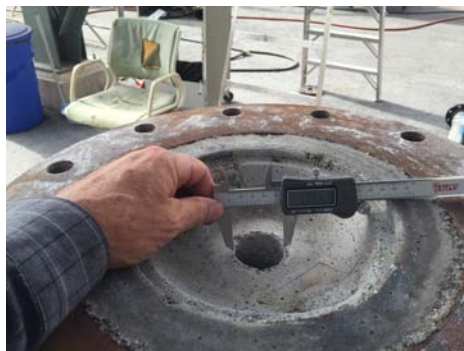
Figure-27. Evaluating Nozzle Erosion
