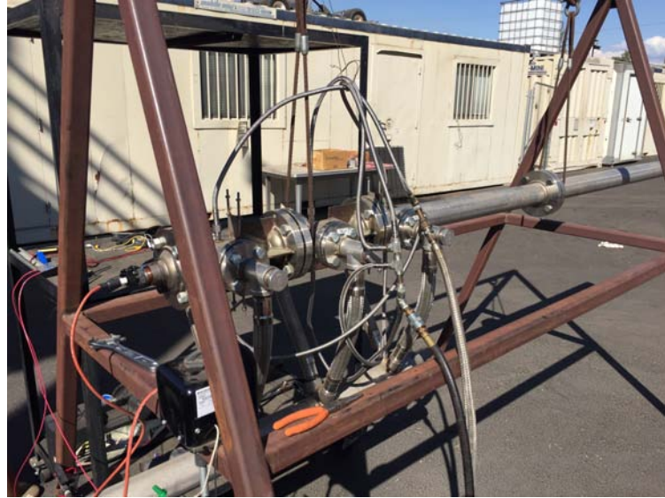
Figure-13. Horizontal test-stand used to measure deflection
